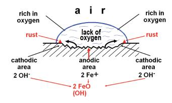
The figure above represents a water drop resting on a plain iron surface. The surface of the water droplet is exposed to air, making it rich in oxygen. The inside of the drop has a lack of oxygen, which creates a difference in electrochemical potential allowing electric current to flow. Electrical current flows through the water, which acts as an electrolyte, from the anodic surface of the iron to the cathodic surface of the water causing iron ions to dissolve.
