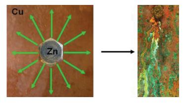
If we reverse the elements and attach a large piece of zinc plated steel with a copper fastener, the current density is very low, and the corrosion process is much more even between the two
